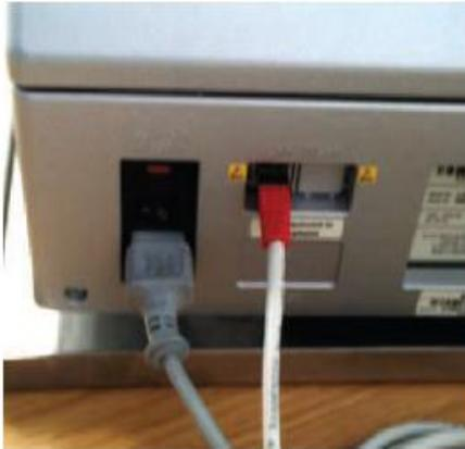
1. Plug a connector of the supplied LAN cable into the LAN socket on the milling unit. The LAN cable supplied is a crossover LAN cable.
