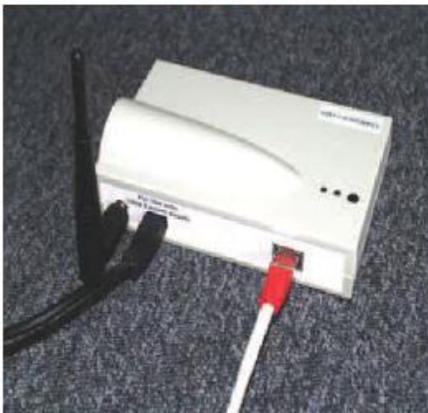
2. Plug the other end of the supplied LAN cable into the LAN port on the radio module.
