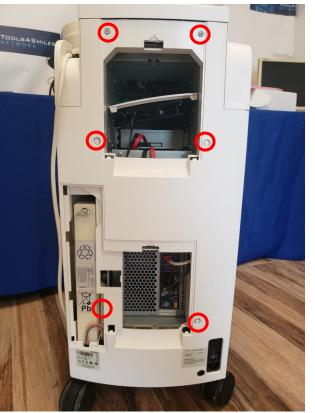
Step 2: Unplug every cord going to the PC. Remove the Circled screws. 4 of them. Now you can slide the PC out using the Handle on the top.
