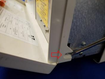
3. Locate Sensor from Pictures below. Clean with –tip/alcohol and Air duster if needed. Run test again.
