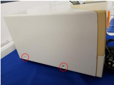
2. Remove front panel (2 screws on the side) Lift rear of front panel over the door
